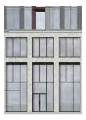
Interface between the base of the building and upper levels of the tower
